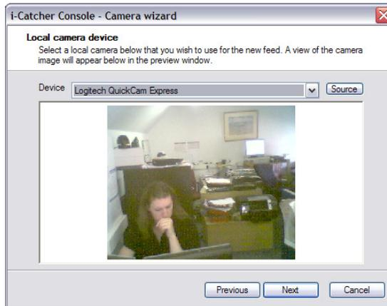
When the device or input is changed, the preview image will update so you can confirm the selected device and input are correct.
